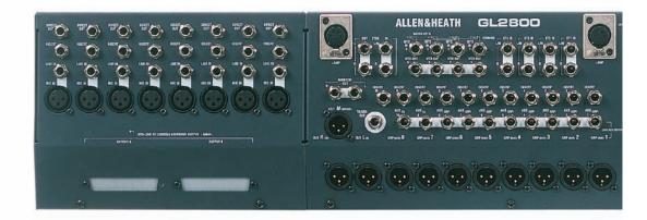
And at the heart of this design is the gain structure allowing a whopping 34dBu maximum input capability and a new ultra-quiet mix head amp section, delivering excellent audio performance.-
